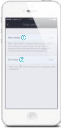
1. When "Alarm delay" is selected, the triggered accessory will sound the Siren when the delay setting times-out. A reminding sound will be heard during this period (the length of the delay can be set by the user). You may activate the delay function in the accessory setting (see pages 24 or 25).
